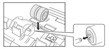
**6** Slide the roller lock lever to the left, and insert it into the retard roller slot.
