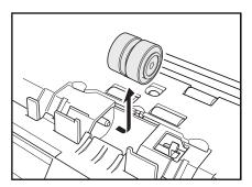
**4** Wipe the removed retard roller with a cloth that has been moistened with water and throughly wrung out.
