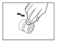
**5** Position the retard roller so the notch in the roller is facing the scanner's shaft.
