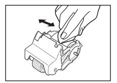
4 Align the cutout on the roller unit with the shaft pin on the main unit.
