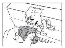
3 Wipe the removed rollers with a cloth that has been moistened with water and thoroughly wrung out.
